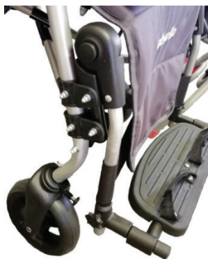
Fig 36. Footrest adjustment mechanism
