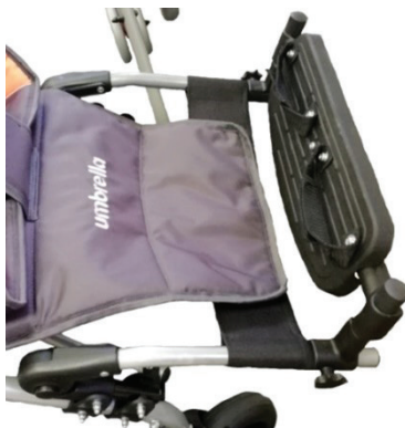
Fig 37. Footrest adjustment mechanism
