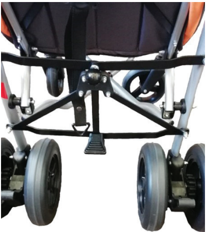
Fig 10. Correct position of rear lock
